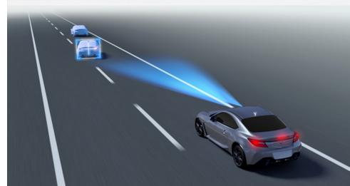
Pre-Collision Braking System\*<sup>5</sup>
